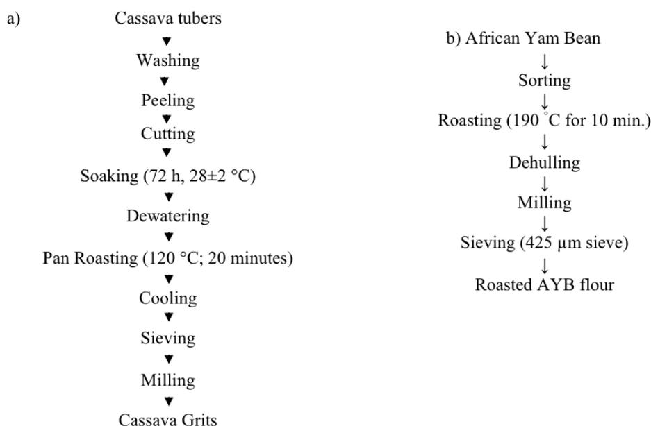
Figure 3: a) Flow chart for the preparation of yellow root cassava grits (Source: Sanni and Jaji (2003); and b) flow chart for the production of AYB flour (Source: Aniedu and Aniedu (2014)).
