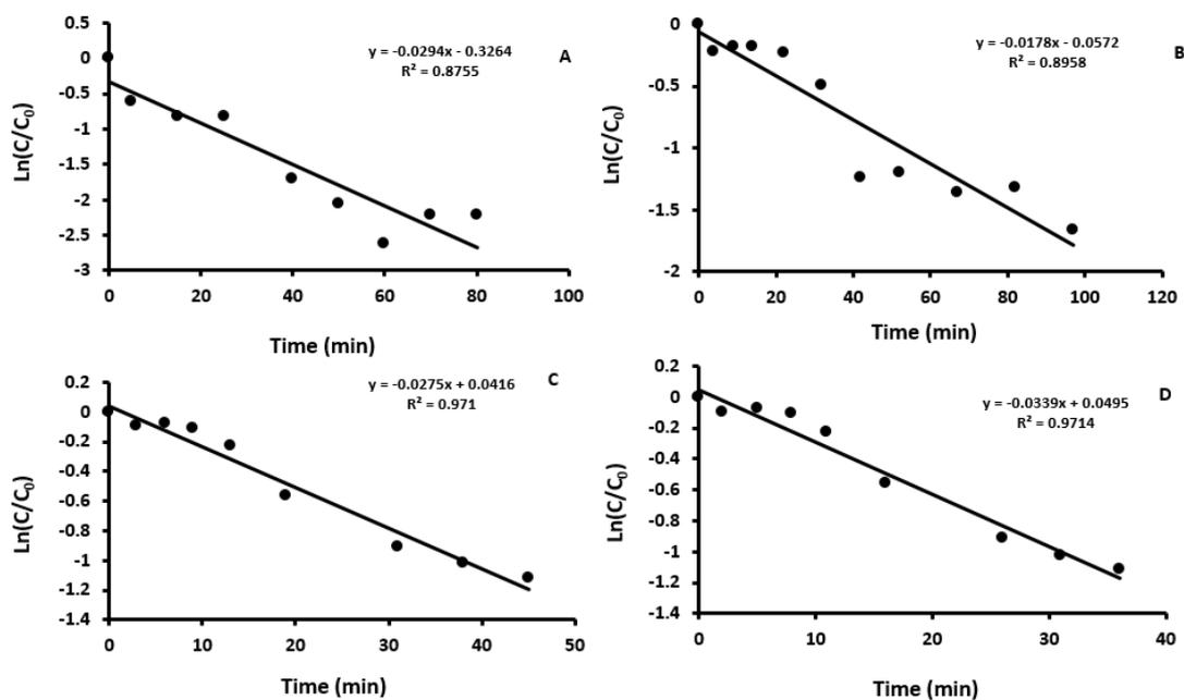
Figure 2: Plots of  $\ln(C/C_0)$  versus time. A: 70°C, B: 80°C, C: 110°C, D: 120°C
