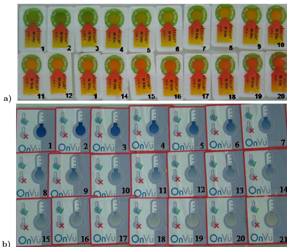
Figure 3: (a) M-type enzymatic TTI label colour scale, (b) B1 photochromic TTI label colour scale)
