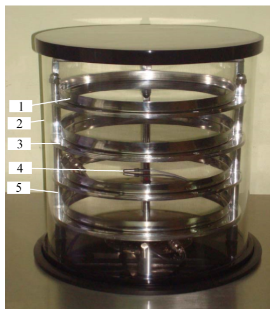
Figure 2: Vacuum chamber of the Rificor L-A-B4-C Freeze dryer. 1. Tray; 2. Transparent vacuum chamber; 3. Temperature-controlled shelf; 4. Product temperature sensor; 5. Framework supporting the structure of the shelves under high vacuum.
